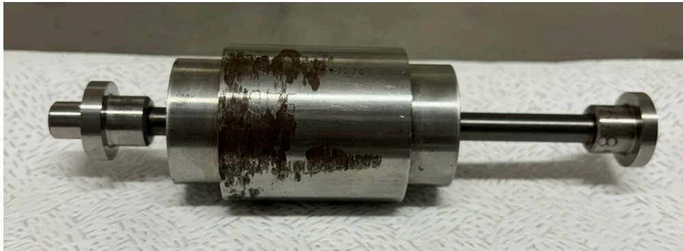
Figure 2) Assembled Punch and die set - 9.8 diameter. The body is made of stainless steel. The ends are of the punches are made of tungsten carbide
